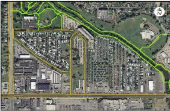
The existing pathways (green) are not connected to the station platform. Creating new pathways (orange) will improve the overall connectivity within the station area.
